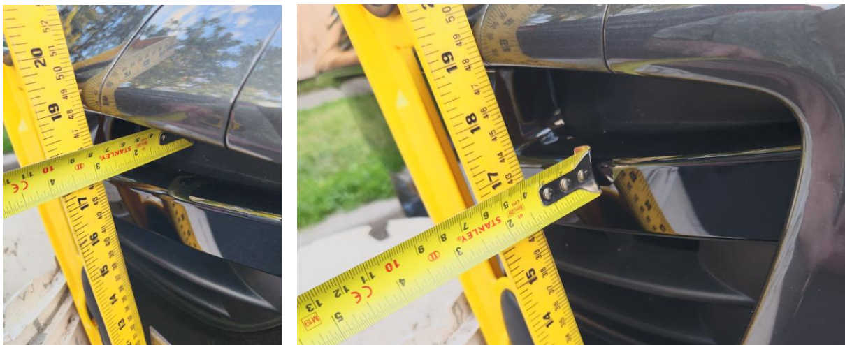
Below the dent area on the leading edge, the bumper is recessed by ~ 2 7/8" & 1 3/8".
